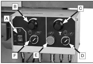
Figure 39. Power feed controls.
